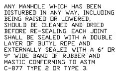
AS WITH NEWLY CONSTRUCTED MANHOLES, ONLY 8" OF ADJUSTING RINGS (2 RINGS TOTAL) ARE ALLOWED. ADAPTOR-SEAL, INFI-SHIELD, CANUSA (WRAPID SEAL) OR APPROVED EQUAL CHIMNEY SEALS ARE REQUIRED IF EXISTING SEAL IS DAMAGED OR DOES NOT EXIST.
