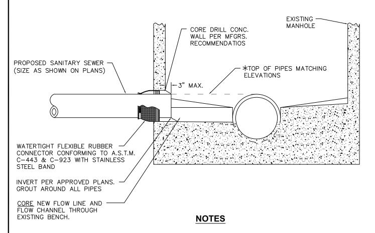
\* TO ESTABLISH THE INVERT OF THE NEW PIPE(S) WHERE THE EXISTING SEWER IS 14" DIA. OR LESS, MATCH THE ELEVATION OF THE TOP OF THE INCOMING PIPE TO THE TOP OF THE EXISTING DOWNSTREAM PIPE. FOR EXISTING SEWERS GREATER THAN OR EQUAL TO 15", SEE APPROVED PLANS.
