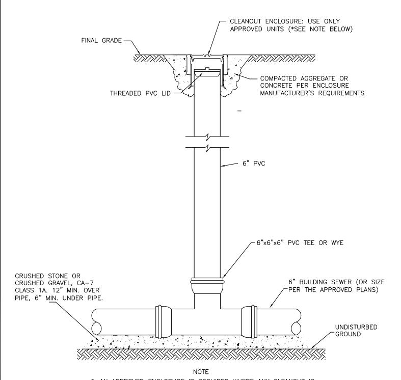
\* AN APPROVED ENCLOSURE IS REQUIRED WHERE ANY CLEANOUT IS INSTALLED WITHIN OR NEAR ANY PAVED SURFACE. IN NON-PAVED AREAS WHERE DAMAGE TO A CLEANOUT MAY OCCUR, ENCLOSURE(S) MAY BE REQUIRED AT THE DISCRETION OF THE DISTRICT.
